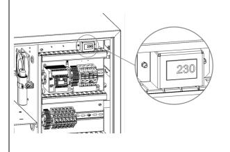
Switch the generator power **ON** at the switch on the front panel.
