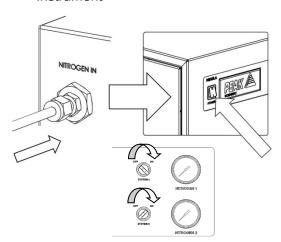
Select the appropriate size Teflon Tubes\*\* and connect to the 'NITROGEN' ports. If using the compression fittings ensure the internal olives are crimped securely.
