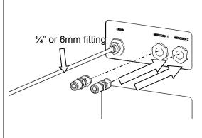
The purge run is now complete. Once the pressure gauge on the front of the generator reads **0** the silencer fittings can be removed from the 'NITROGEN' ports.
