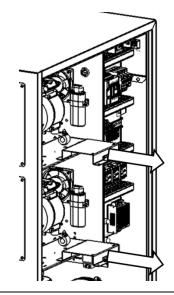
Repeat steps 4 and 5 to remove the LH transit brackets located under both of the LH compressors. These will pull out in the same way.
