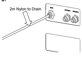
From the fittings kit, select one of the 6mm push-fit fittings and connect it to the port marked '**DRAIN**' on the rear of the unit using a 16mm or 5/8" spanner.
