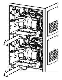
With the RH side panel removed you now have access to the RH transit brackets. These are located under both of the RH compressors and are painted red. To remove the transit brackets remove the 4 screws on each bracket as indicated.
