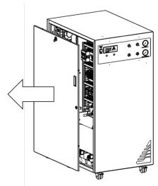
Remove the LH side panel as before, taking care to disconnect the earth lead located on the inside of the door panel.
