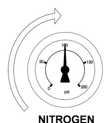
The 'NITROGEN' pressure gauge on the front of the generator will again gradually increase from 0 to 100psi as the pressure in the internal storage tanks increases.
