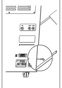
Unpack the generator from the shipping crate and place on a flat surface. To remove the transit brackets, firstly remove the RH side panel.
