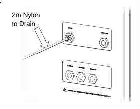
From the fittings kit, select the 6mm push-fit fitting and connect it to the port marked 'DRAIN' on the rear of the unit using a 16mm or 5/8" spanner.
