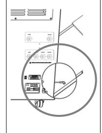
Unpack the generator from the shipping crate and place on a flat surface. To remove the transit brackets, firstly remove the RH side panel.
