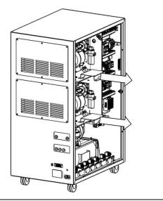
Repeat steps 4 and 5 to remove the LH transit brackets located under both of the LH compressors. These will pull out in the same way.
