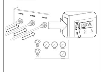
Select the appropriate size Teflon Tubes\*\* and connect to the 'CURTAIN' 'SOURCE' 'EXHAUST' & 'NITROGEN' ports. Ensure the internal olives are crimped securely, within the compression fittings
