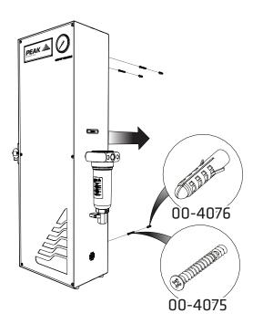
With the holes drilled in your desired location, fit the  $3 \times 10.8$  Wall Plug 00-4076 and  $3 \times 10.8$  Screw 00-4075 to the wall and mount your generator onto them.
