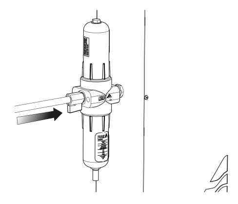
Attach your house air supply to the **BA filter** at the **left side** of the generator. Ensure the valve on the filter is at the **open** position.
