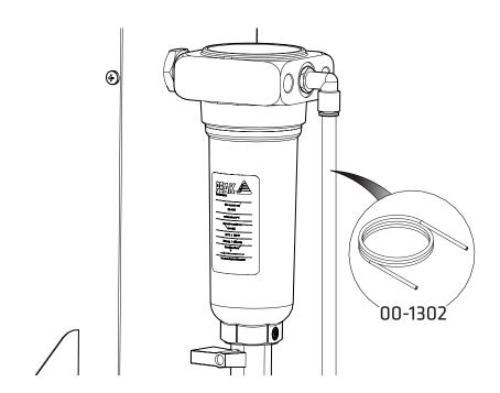
Attach the supplied **6mm OD Teflon 00-1302** and connect this to the **1/4" - 6mm Push Fit Elbow Fitting 02-4331**.
