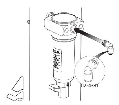
Select the 1/4" - 6mm Push Fit Elbow Fitting 02-4331 and attach it to the filter outlet on the right side of the generator. It is recommended that PTFE tape is applied to the threads to ensure a leak-tight fit.
