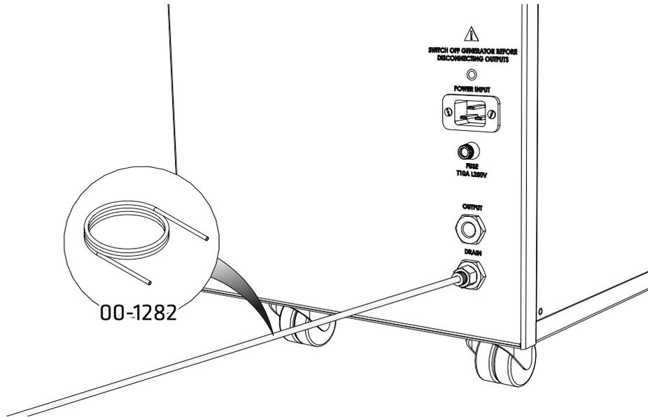
Connect the **6mm PE Tubing 00-1282** to the  $\frac{1}{4}$ "- **6mm Push Fit Fitting 02-4600**.
