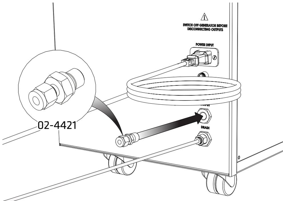
Depending on the size of the inlet on the instrument, select either the ¼" **Compression Fitting 02-4421** or the remaining ¼"- **6mm Push Fit Fitting 02-4600** and attach this to the **Nitrogen port**.
