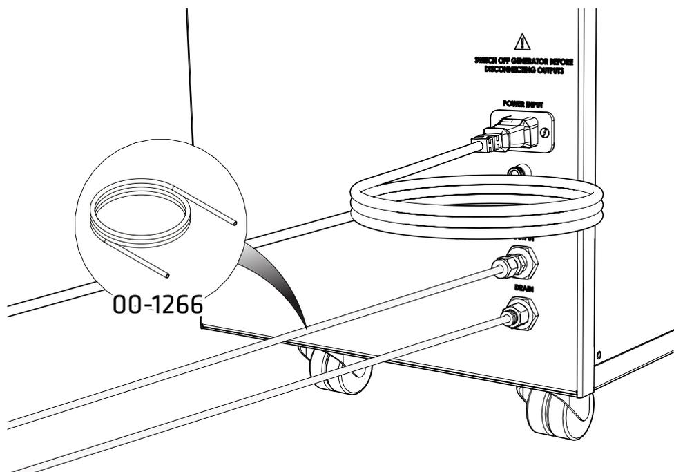
Attach the appropriate sized **Teflon tubing** to the fitting attached to the **nitrogen port** and connect to the **gas inlet of your instrument**.
