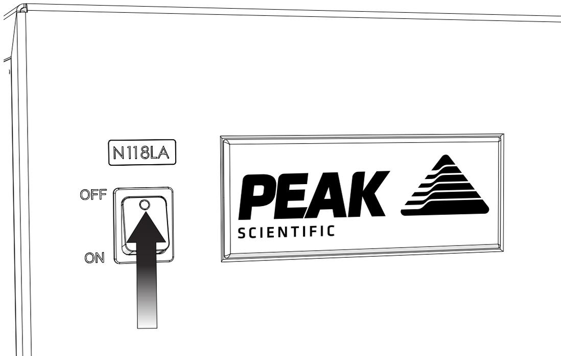
Switch the generator **ON** using the switch on the front panel.
