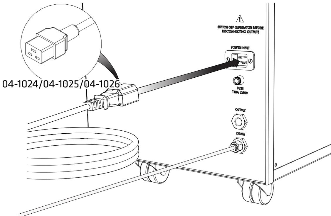
Select the appropriate mains cable from the fittings kit and plug the **IEC 60320/C19** cable into the mains input at the rear of the generator.
