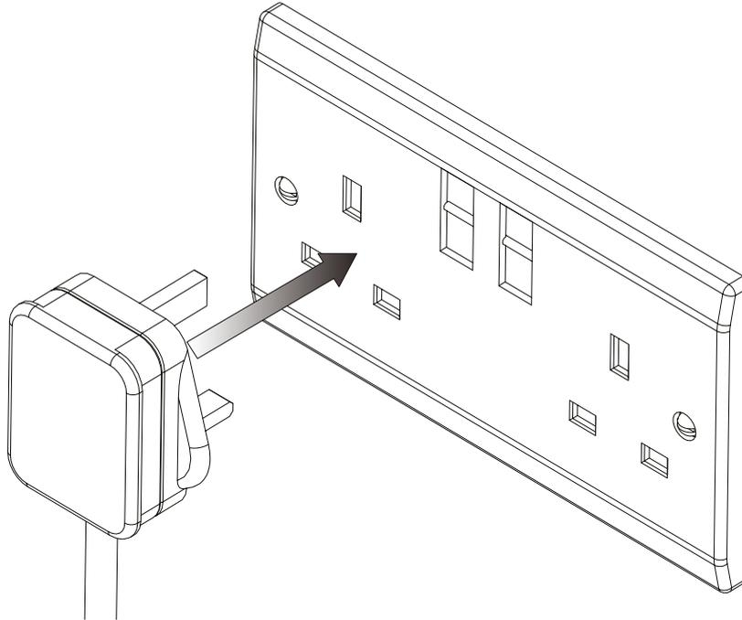
With the side panels securely re-attached, the mains power supply can be **re-connected**.
