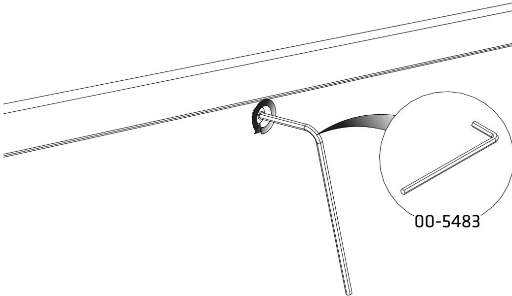
Using a **2.5mm Hex Key 00-5483** remove each screw by turning anti clockwise.
