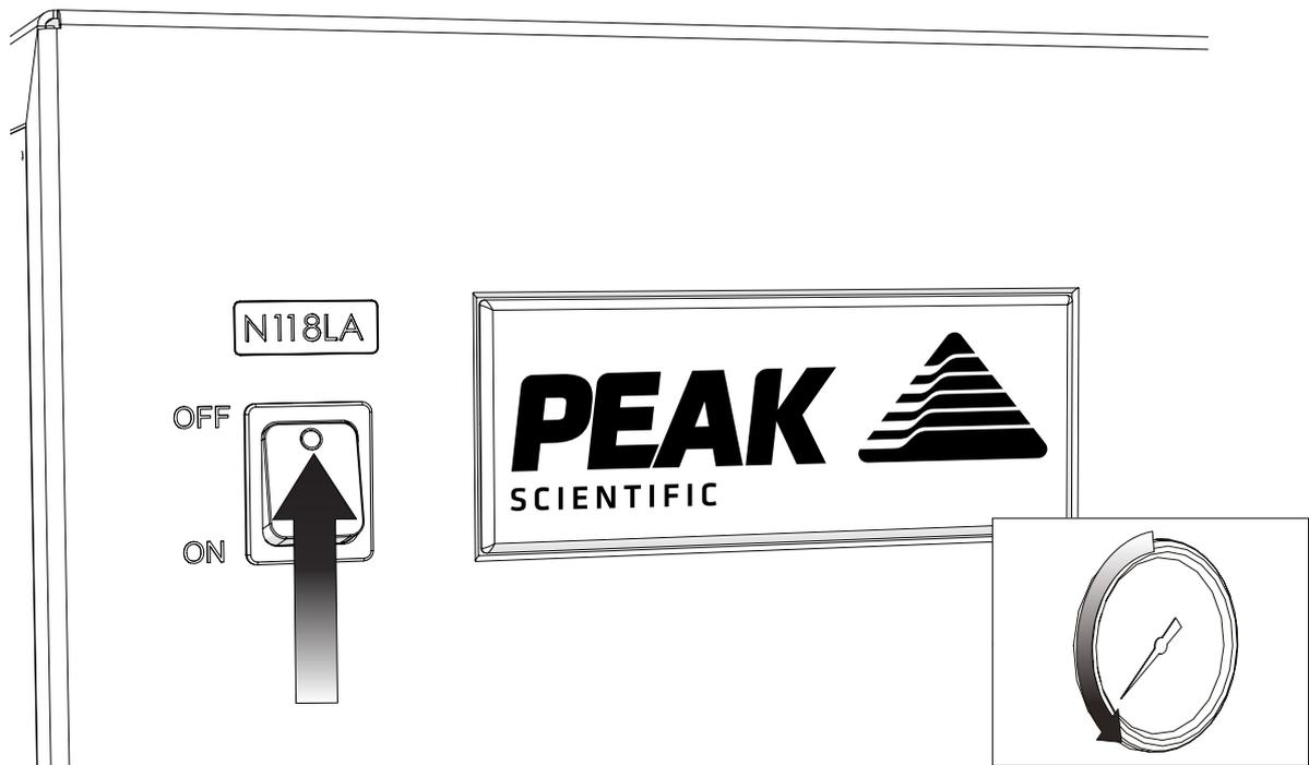
The purge is now complete, switch the generator **OFF** using the switch on the front panel. Once the **pressure gauge** reads **0**, the installation can continue.
