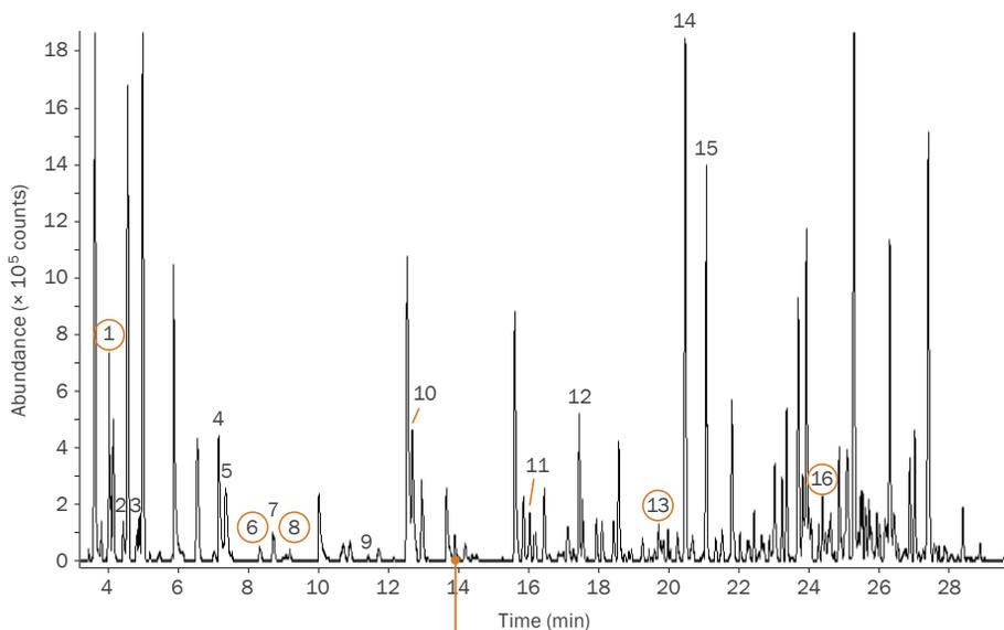
**The simultaneous detection of acetaldehyde, styrene and sulfur species** (circled) in this sample of landfill gas illustrates the ability of Markes' TD systems to analyse a wide compound range in one run.
