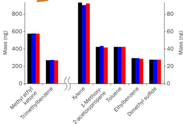
**Method-compliant, quantitative analysis of high-concentration stack gas** is confirmed by re-collecting the split sample onto a clean sorbent tube, followed by re-analysis.
