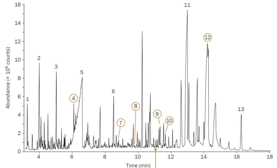
**A range of sub-ppt SVOCs** – including analytically challenging PAHs (circled) – are detected in this Chinese urban air sample, as well as typical 'air toxic' VOCs.
