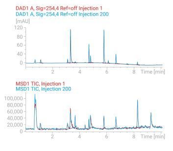
Our LC/MS instruments deliver superior reproducibility of retention time, peak area, peak resolution, and mass accuracy. Here we show data for repeat injections on an LC/MS single quadrupole system.
