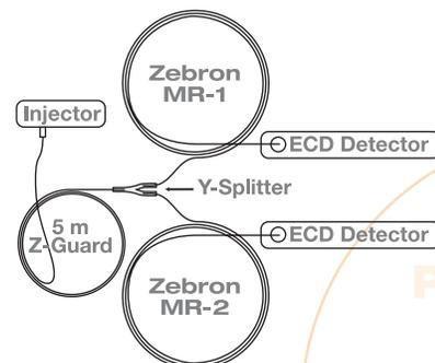
By making one injection and splitting the sample into two columns, both Procedure A and Procedure B can be accomplished at the same time. If a calibration curve is run before each batch of samples and a suitable calibration check is run after each batch of samples to verify the stability of the calibration, then Procedure C could also be run at the same time. The main obstacle of using this type of system is to use one oven program to separate the target analytes on two column phases.
