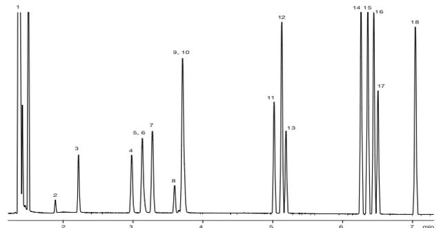
Figure 3 shows the separation of 18 solvents from Class 1, 2, and 3 using a G16 equivalent phase. Column length and internal diameter were chosen to achieve maximum resolving power with minimal analysis time. Choosing these conditions allowed the method to be completed in less than 8 minutes with a total cycle time of less than 10 minutes.
