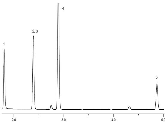
**Figure 3.** Separation of 18 solvents from Class 1, 2, and 3 using a G16 equivalent phase.
