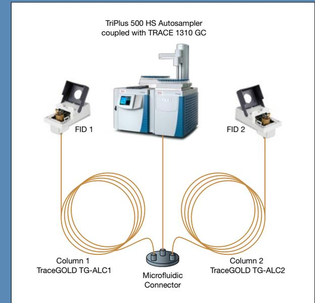
Dual-FID configuration implemented through a microfluidic connector
