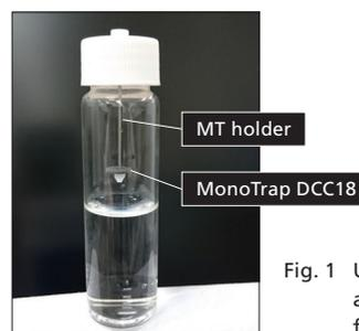
Fig. 1 Using a MonoTrap adsorbent to trap fragrance components
