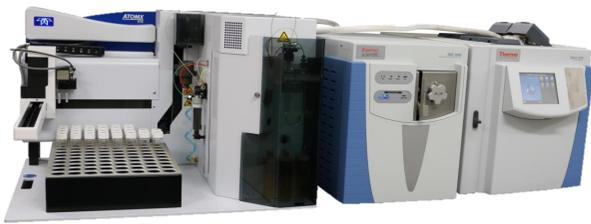
Figure 1. Teledyne Tekmar Atomx XYZ P&T coupled to the ISQ 7000 AEI GC-MS
