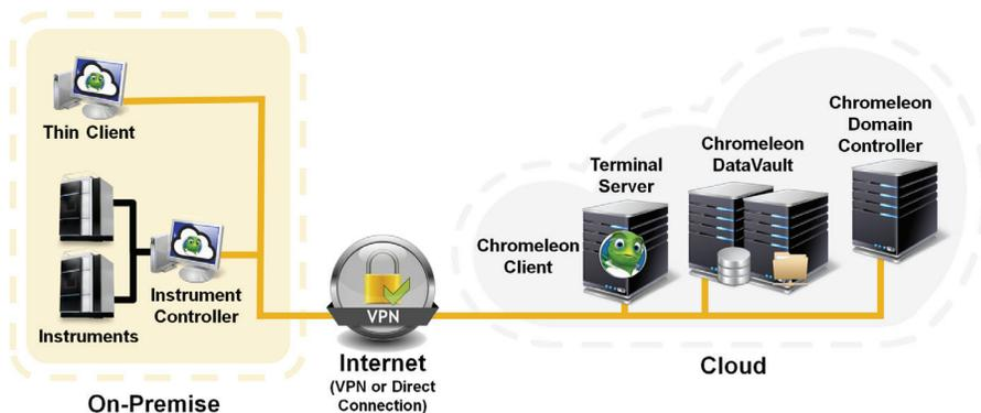
Figure 4. Chromeleon CDS Thin Client Cloud Deployment Example
