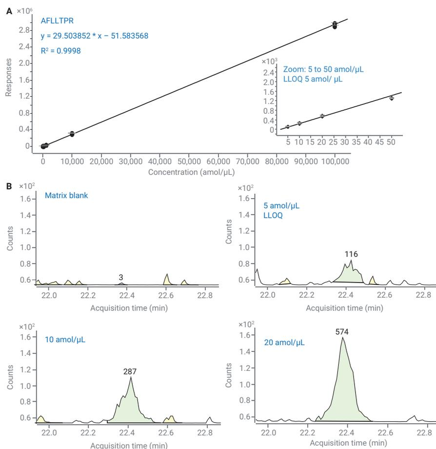
Figure 1. Quantitative performance of the SIS peptide AFLLTPR from apolipoprotein M in plasma. (A) standard curve of SIS peptide AFLLTPR for the range from 5 amol/μL to 100 fmol/μL in 1 μg/μL plasma digest with inset showing detail for the range of the curve from 5 to 50 amol/μL. (B) extracted ion chromatograms for peptide AFLLTPR showing the LLOQ.
