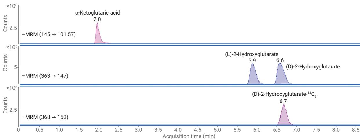
Figure 1. Standard MRM chromatograms representing the separation of (D) and (L)2-HGA, D-2-HGA-<sup>13</sup>C<sub>5</sub>, and αKG.
