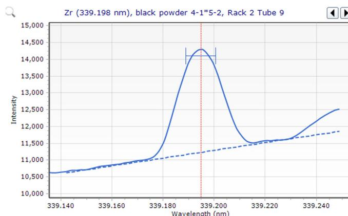
**Figure 2.** Automatic background fitting for Zr 339.198 nm using FBC.
