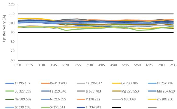
**Figure 5.** Stability of the Agilent 5800 VDV ICP-OES during the analysis of 198 solutions run over seven hours, with no recalibration and no internal standard correction. The CCV QC sample was analyzed every 10 samples.
