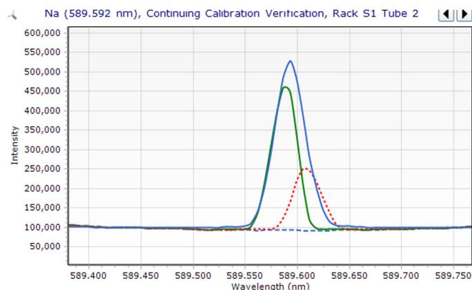
**Figure 3.** FACT model for correction of a Ba interference on Na (shown in blue). The Ba 589.612 nm (red dashed) interference line is overlapping the Na 589.592 nm (green) line. The light blue dashed line represents the blank.
