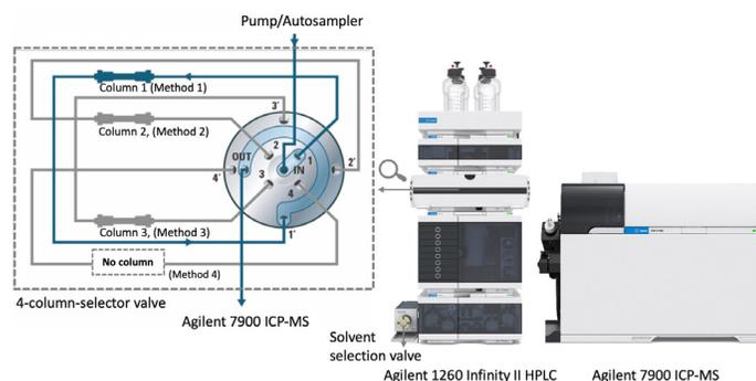
**Figure 1.** Schematic of the HPLC-ICP-MS system with Quick Change valve head used in this study. The 4-column-selector valve head and quaternary pump enabled automated selection of the different HPLC columns and solvents.
