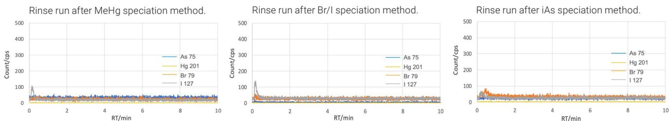
**Figure 7.** Background signals in wash methods confirm minimal carryover between analytical method runs on day 2.
