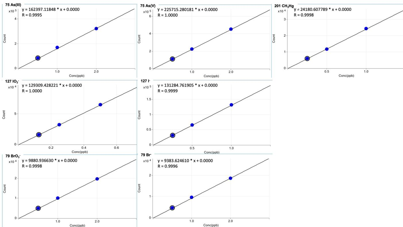
**Figure 4.** Calibration curves showing excellent linearity. Top: As (III), As(V), and CH<sub>3</sub>Hg; Middle: IO<sub>3</sub><sup>-</sup> and I<sup>-</sup>; Bottom: BrO<sub>3</sub><sup>-</sup> and Br<sup>-</sup>.
