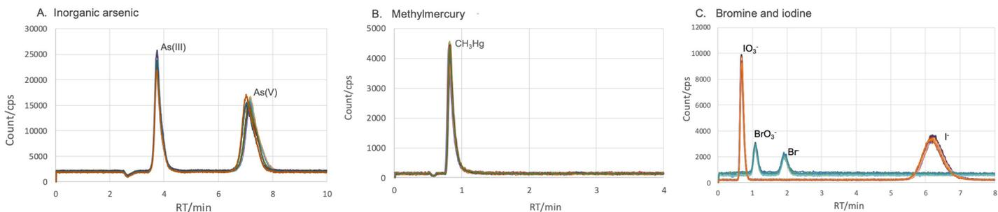
**Figure 5.** Overlaid chromatograms of A: inorganic arsenic, B: methylmercury, and C: bromine and iodine species obtained from nine injections of level-3 calibration standards. Shows excellent stability of retention times and peak areas over three days. n=9 for each chromatogram.
