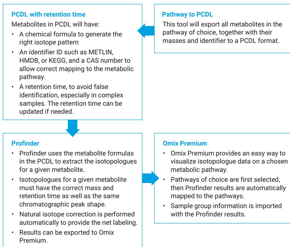
**Figure 1.** Overview of VistaFlux data analysis workflow.
