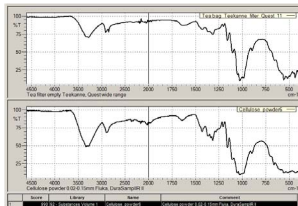
Fig. 4: search result of the filter in the library collection, Cellulose was found with a match of 990. Score maximum is 1000.
