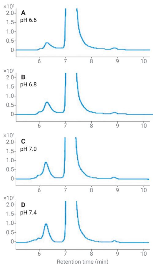
**Figure 1.** Size exclusion chromatograms of NIST mAb using  $4.6 \times 300$  mm SEC columns running at 0.35 mL/min under 150 mM sodium phosphate at A) pH 6.6, B) pH 6.8, C) pH 7.0, and D) pH 7.4.
