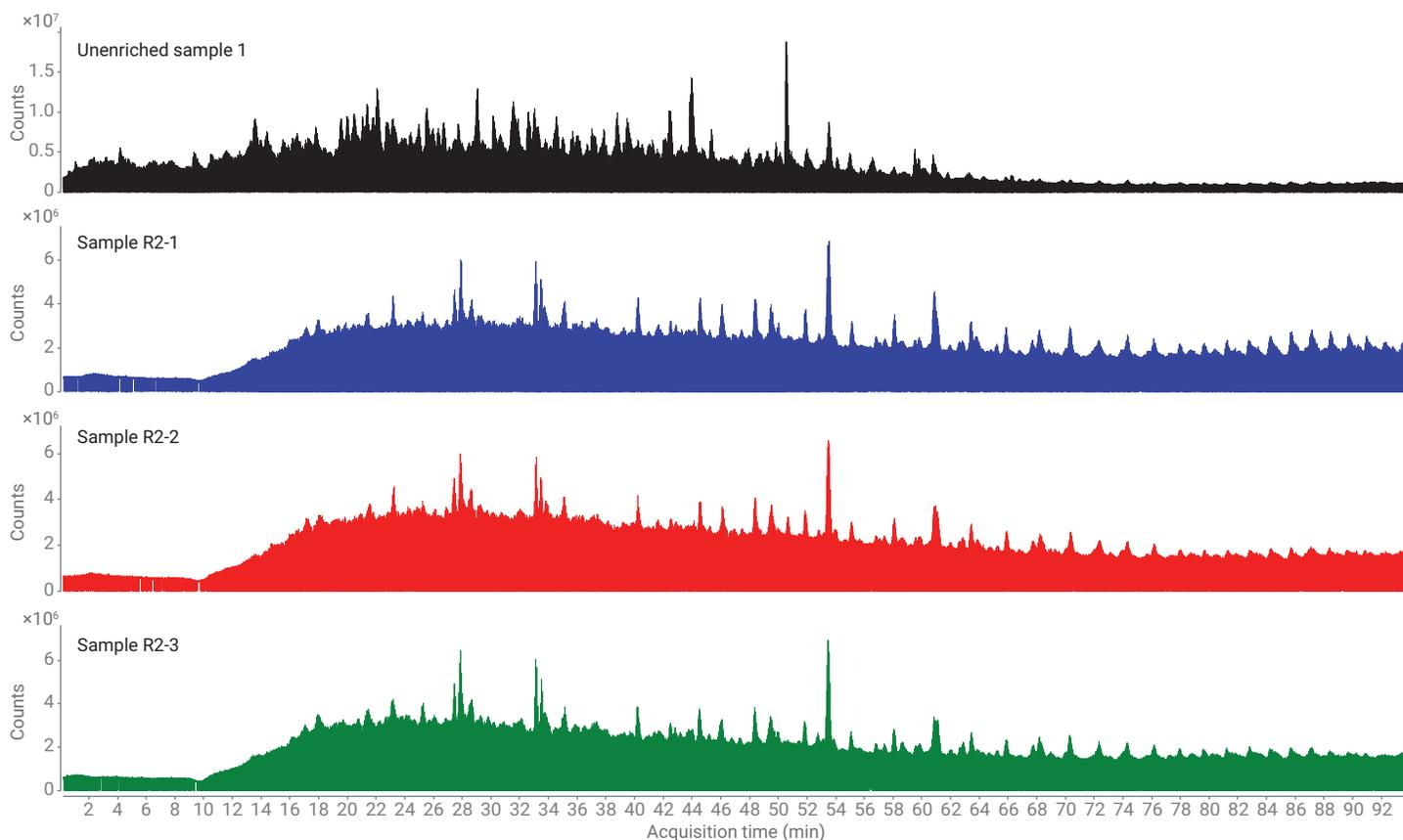
**Figure 5.** TIC of unenriched sample compared to enriched sample R2 using a 90-minute LC gradient.
