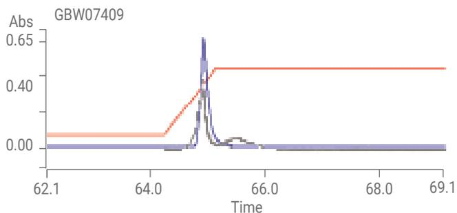
**Figure 1.** The signal generated by total Pb in 10 μL of the digest of reference soil material GBW07409 on Agilent 280Z graphite furnace atomic absorption spectrometer.
