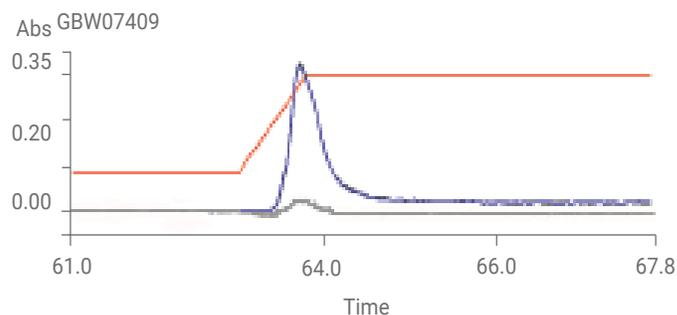
**Figure 2.** The signal generated by total Cr in 10 μL of the digest of reference soil material GBW07409 on Agilent 280Z graphite furnace atomic absorption spectrometer.
