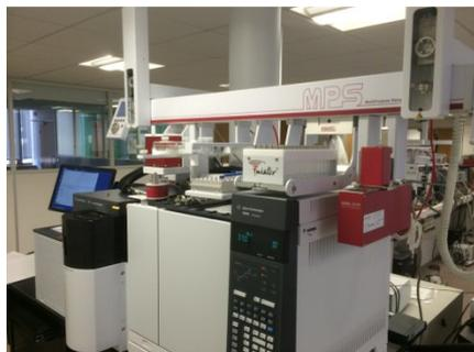
Figure 2: Photo of Multiflex GC/Q-TOF
