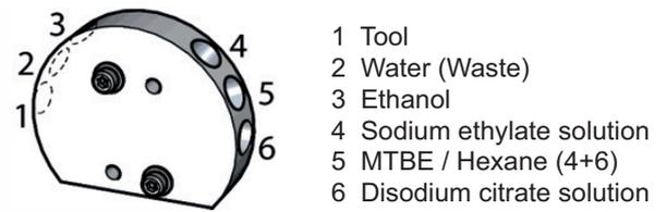
Fig 4: Up to 5 different solvents and solutions may be dispensed by the dilutor tool.
