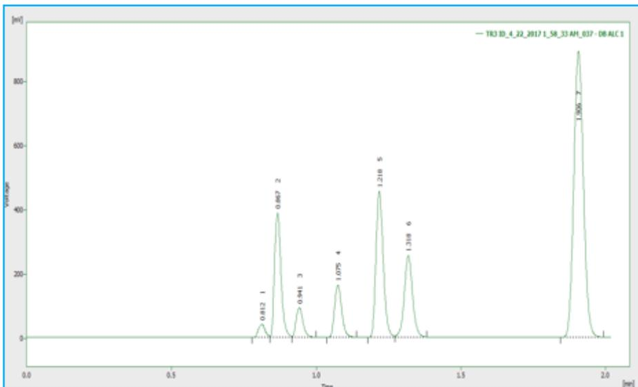
Figure 1: Resolution mix on DB-Alc1
