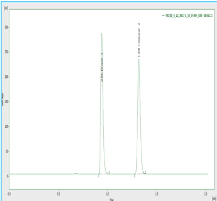
Figure 2: Typical BAC chromatogram of ethanol and n-propanol ISTD
