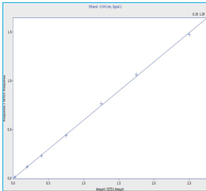
Figure 3: ethanol 7- point calibration curve 0.005% - 0.5% ethanol on DN-Alc1, He
