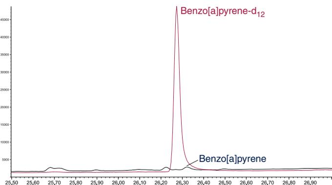
Figure 10. Benzo[a]pyrene in sample E, SIM, m/z 252; 264.
