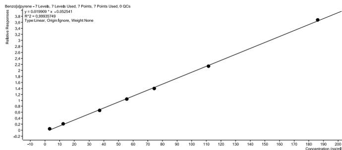
Figure 12. Calibration curve for benzo[a]pyrene, 3.1-186 ng/mL.
