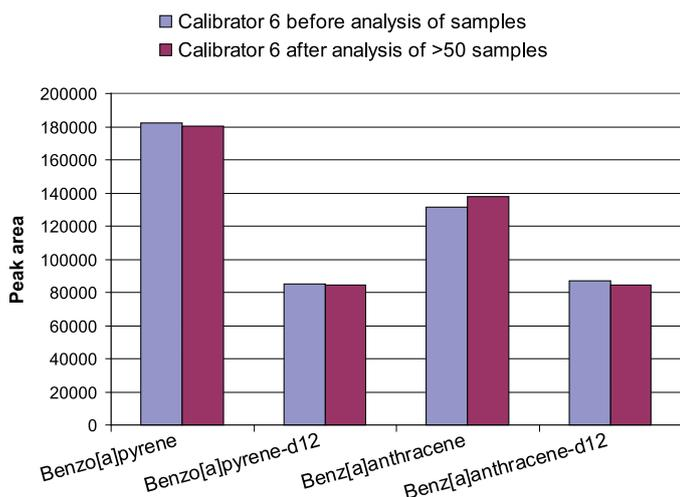
Figure 17. Peak areas for calibration standard 6 remain constant even after analysis of more than 50 samples.
