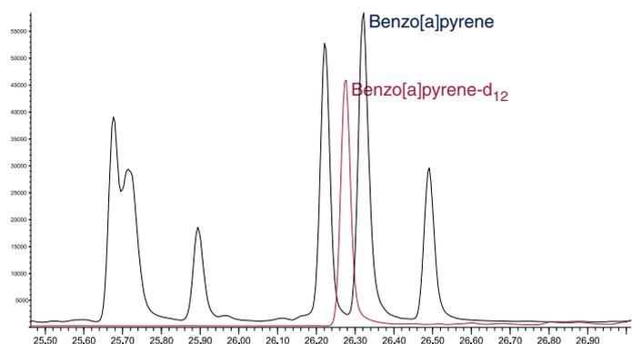
Figure 7. Benzo[a]pyrene in sample B, SIM, m/z 252; 264.
