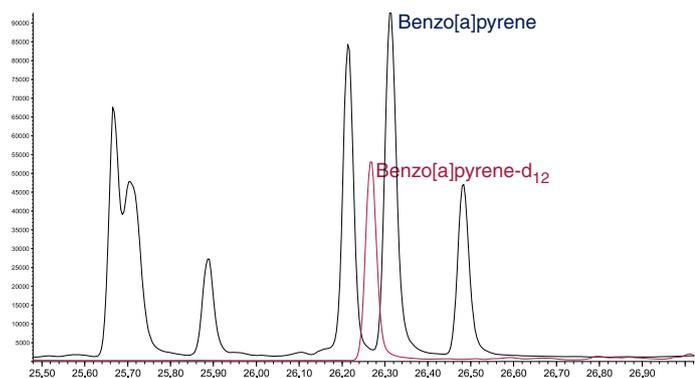
Figure 6. Benzo[a]pyrene in sample A, SIM, m/z 252; 264.
