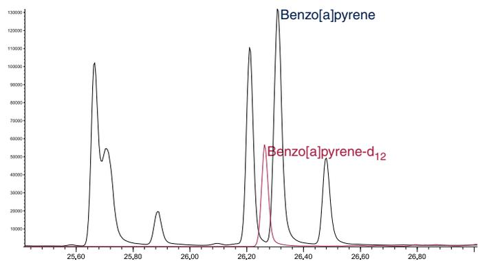
Figure 8. Benzo[a]pyrene in sample C, SIM, m/z 252; 264.
