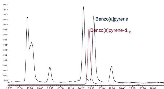
Figure 9. Benzo[a]pyrene in sample D, SIM, m/z 252; 264.
