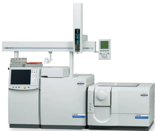
Bruker 300-MS triple quadrupole mass spectrometer with 450-GC gas chromatograph and CTC Combi PAL™ autosampler.
