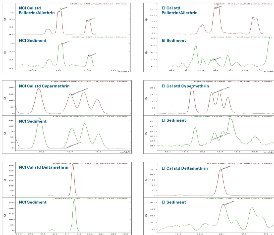
Figure 5: Comparison of NCI (left) and EI (right) extracted ion chromatograms for (top to bottom) Allethrin/Pallethrin, Cypermethrin isomers, Deltamethrin.
