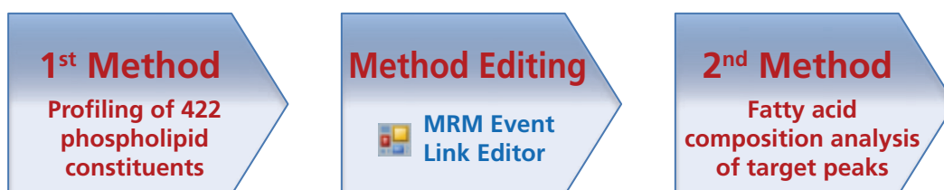
Fig. 2 Workflow of MRM based phospholipid profiling. Structural information obtained from the 1 st method comprises the polar head group, and the total carbon number of the fatty acids and number of double bonds (eg: PC (34:1)). The 2 nd method is used to determine the fatty acid composition of the constituent obtained in the 1 st method, such as PC (16:0/18:1) from PC (34:1).
