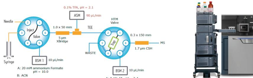
Figure 1. Fluidic configuration for two-dimensional high pH/ low pH RP/RP chromatography, employing pre-trap on-line dilution.
