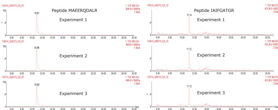
Figure 2. LC separation reproducibility of the 2DLC chromatographic system. Extracted mass chromatograms were generated for the monoisotopic peaks of two low-abundance HCP peptides. The peptides reproducibly elute in the same fraction at consistent retention times over the course of the triplicate HCP discovery experiment.
