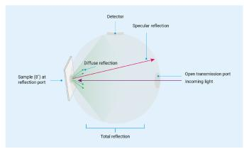
Schematic showing how reflectance measurements are performed using the Agilent Cary 60 UV-Vis DRA. The sample is mounted at the reflection port of the DRA, ensuring efficient collection of the diffusely reflected light (green). Although commonly referred to as a "diffuse reflectance accessory", the DRA allows users to exclude or include the specular component of reflected light, providing the flexibility to choose between diffuse-only or total reflectance measurement modes.
