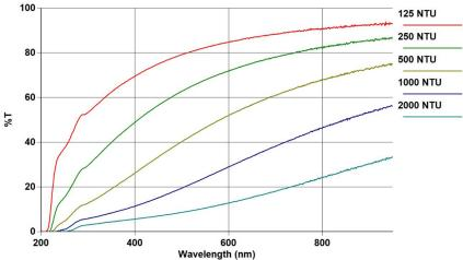
Diffuse transmission of formazin standards (125 to 2000 NTU (= Nephelometric Turbidity Unit)) measured using the Agilent Cary 60 UV-Vis DRA to assess light scattering behavior. Each measurement was performed using the standard 10 mm cuvette holder. Formazin is widely used to assess turbidity in water quality testing and to evaluate clarity of juices, beers, and dairy products, where haze formation can impact product quality.
