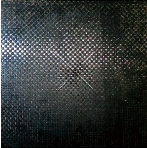
Fig. 4 Surface image of CFRP with conductive polymer matrix subjected to a lightning strike (X indicates the lightning entry point)
