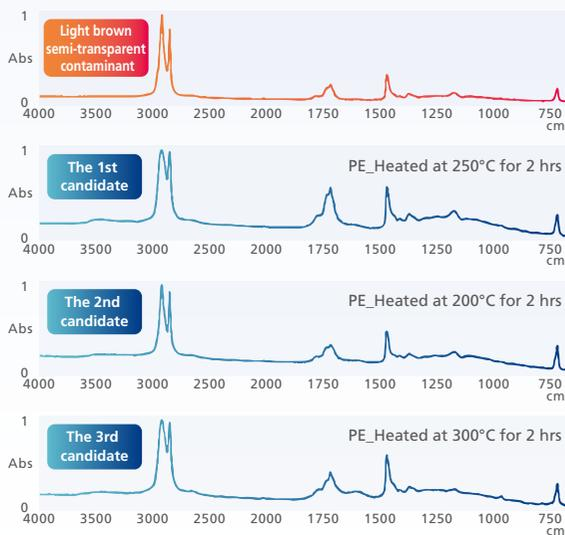
The measurement of a light brown semi-transparent contaminant on a plated item was performed. The figure above shows that the spectral pattern of the acquired infrared spectrum differs from the standard polyethylene (PE).
