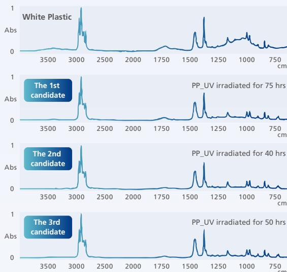
The top right figure shows the search results from measurements by Plastic Analyzer of a white plastic (PP material) that was left outdoors for an extended period and exposed to UV rays.
