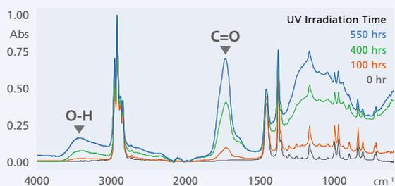
Plastics degrade as they experience molecular cleavage and cross-linking due to heat and light. As a result, in fault analysis and failure analysis, the qualities of deteriorated samples must be analyzed. The above left figure shows the infrared spectrum of a polypropylene (PP) sample that has been irradiated with UV rays. The UV irradiation has caused the plastic to deteriorate, and it is evident that the shape of the infrared spectrum has changed.
