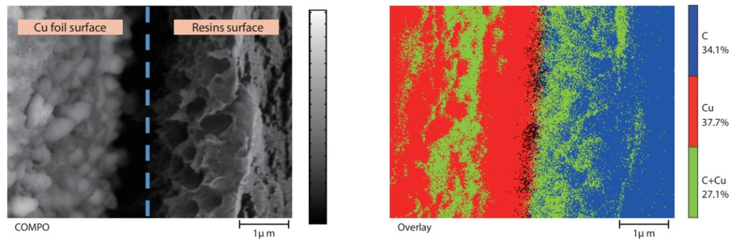
Analysis of Printed Circuit Boards for 5G Communication Equipment
