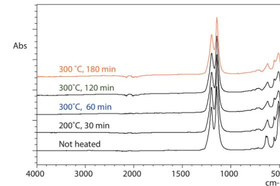
Property Evaluation of Fluorocarbon Resin Supporting Popularization of 5G by FTIR and TGA
