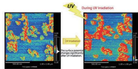
Fig. 1. a Surface Potential Before UV Irradiation. The average potential difference between the glass substrate and the catalytic particles is 200 mV. Fig. 1. b Surface Potential During UV Irradiation. The average potential difference between the glass substrate and the catalytic particles is 330 mV.
