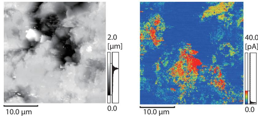
SPM (AFM) Measurements of Cathode and Anode Materials from All-Solid-State Lithium-Ion Batteries without Exposure to Air
