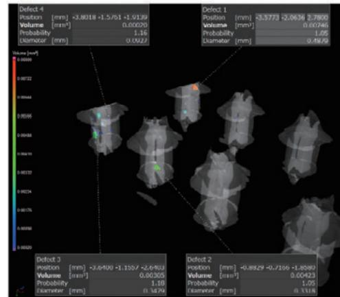
Observation of an Automotive Computer Using the inspeXio SMX-225CT FPD HR X-Ray CT System
