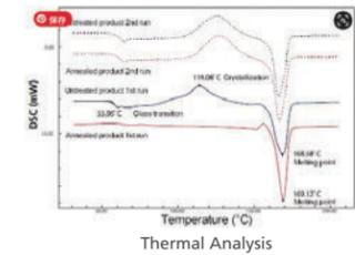
The results showed that the mechanical properties changed due to crystallization.
