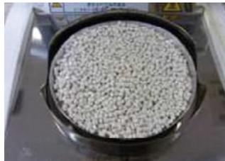
Fig. 8 Plastic Pellets on the Moisture Analyzer after Drying
