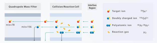
Note: Example of how reaction mode can be used. Reaction gas  $H_2$  is used in this example to convert doubly-charged ions to singly-charged ions, and charged polyatomic ions to neutral clusters.
