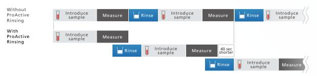
Note: The reduction in time depends on the measurement conditions. In the example above, the Preset method for Drinking Water in ICPMS-2040 was used.
