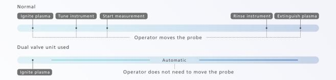
When using an Online Internal Standard Kit (optional), the operator must move the probe before and after data acquisition. The optional Dual Valve Unit allows seamless switching between tuning solution and rinsing solution while also automatically adding internal standard solution to samples. The entire sequence, from instrument tuning, to measurement, to rinsing, and plasma off, are performed automatically.
