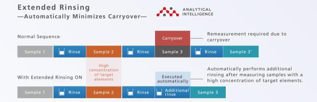
Analyzing samples containing a high concentration of target elements can cause carryover to the next sample, preventing accurate measurements. The extended rinsing function automatically performs an additional rinse sequence when a target element exceeds a predetermined upper limit. A second rinse solution can be used in the additional rinsing sequence to improve rinsing effectiveness. Consequently, carryover is eliminated to ensure high-quality data.
