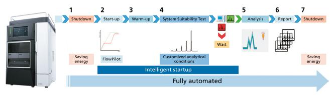
Fig. 5 Workflow Diagram showing the Fully-automated Operation of LC Analysis
