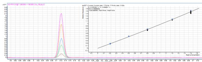
**Figure 2: Overlaid chromatogram of pp-DDT at 20, 50, 80, 120 and 150 ng/L in solution**
