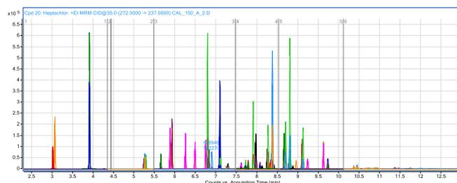
Figure 1: Extracted MRM transitions of all pesticides at 150 ng/L
