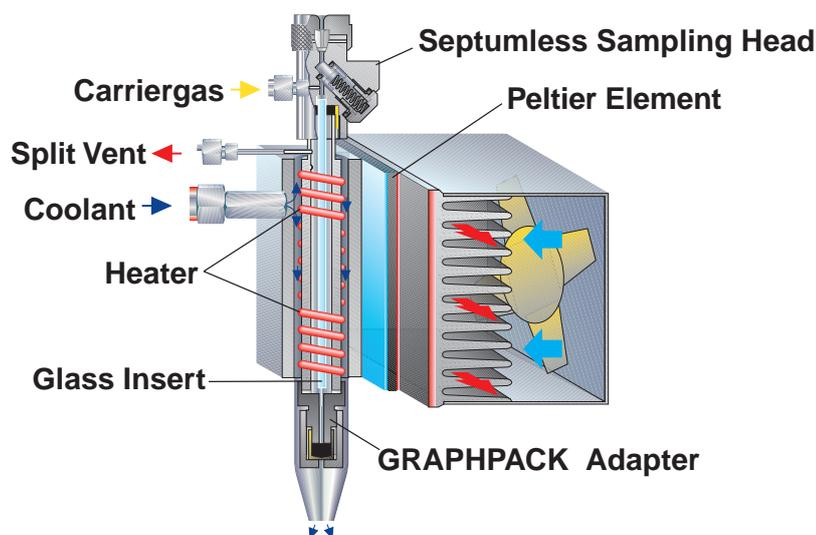
**Figure 2.** Gerstel Cooled Injection System CIS 3.
