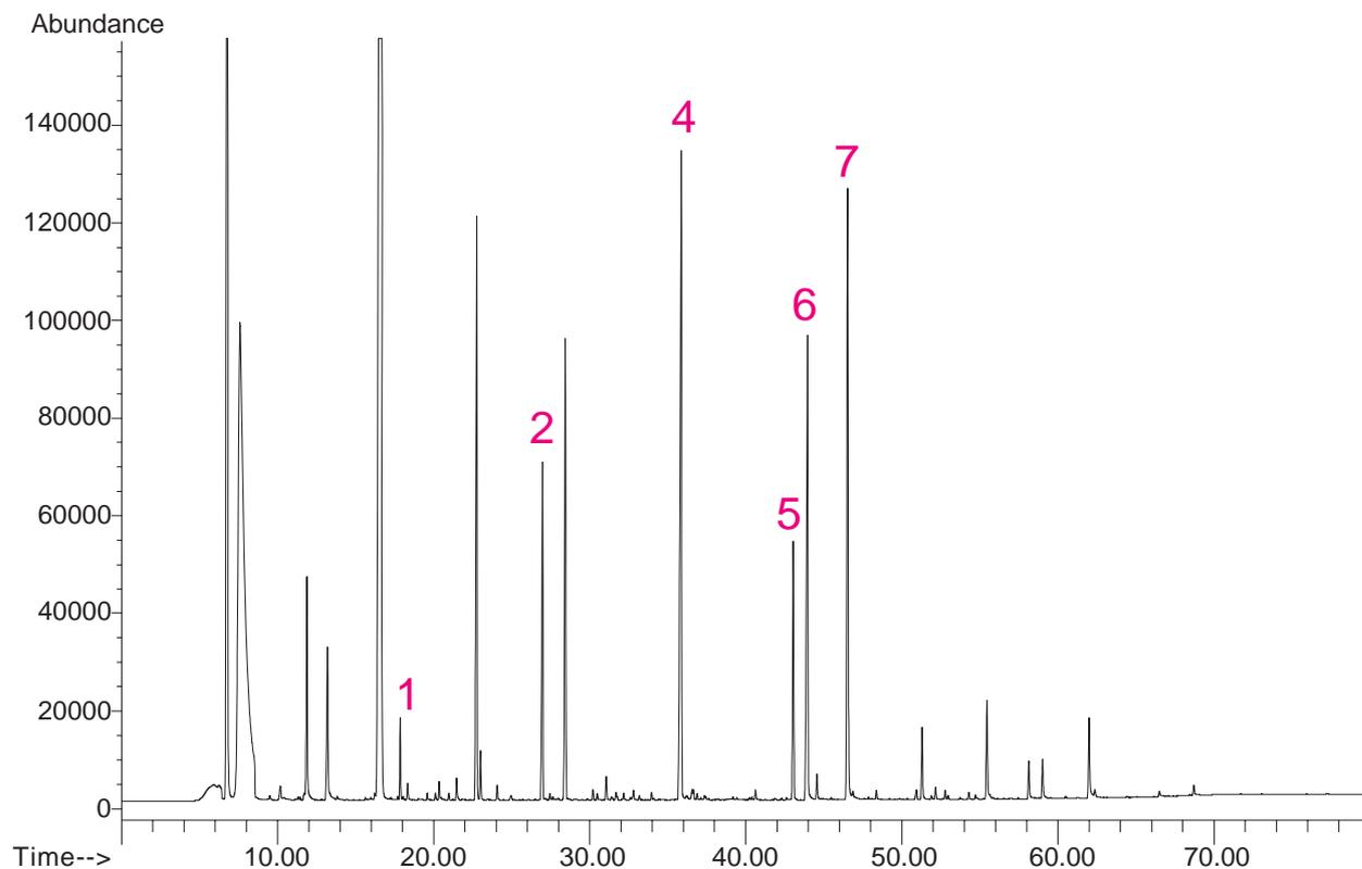
**Figure 4.** FID chromatogram of a 10  $\mu$ l injection of a whiskey, compound identification see table I.
