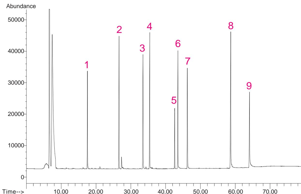
**Figure 3.** FID-chromatogram of a 50 µl injection of a test-mix, compound identification see table I.
