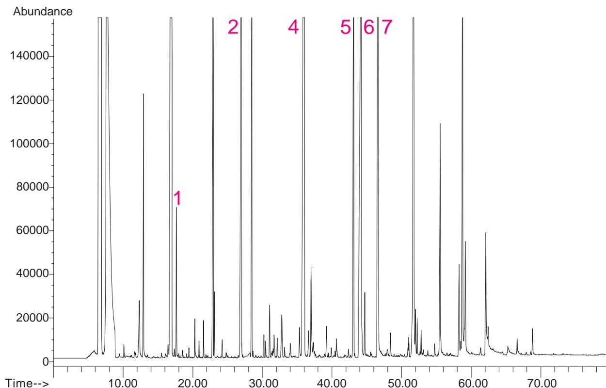
**Figure 6.** FID chromatogram of a 50 µl injection of a whiskey, compound identification see table I.
