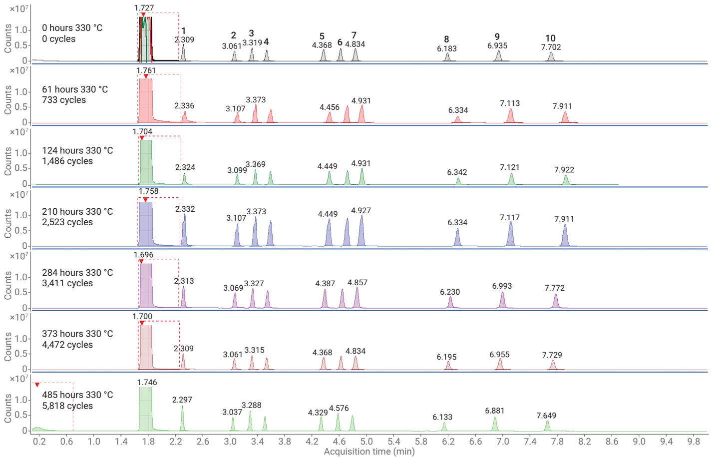
**Figure 2.** The J&W VF-5ms Intuvo column 5 was tested with test mix 82, and showed stable performance (inertness and separation) over the course of the lifetime test (485 hours at 330 °C, 5,818 cycles).
