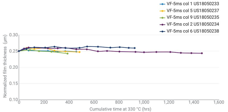
**Figure 3.** Film thickness stability of J&W VF-5ms Intuvo GC columns (n = 5) tested after cycling to 330 °C for several hours.
