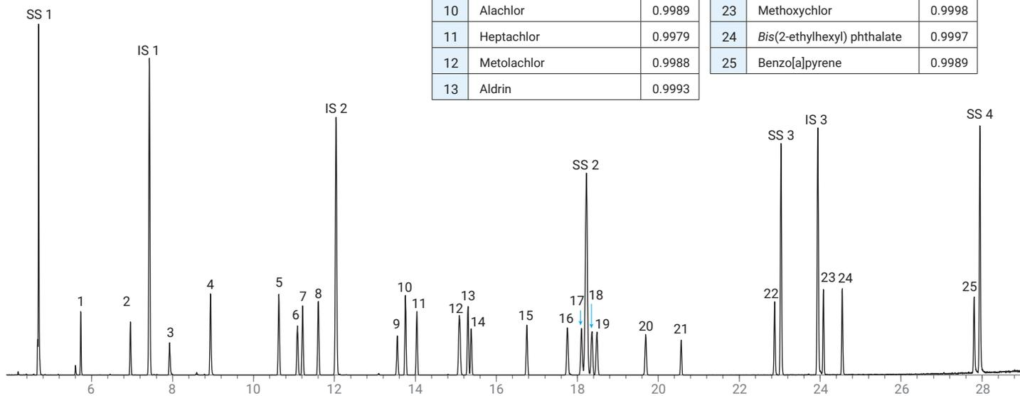
Figure 5. TIC of the regulated semivolatile mixture using a J&W VF-5ms Intuvo GC column.
