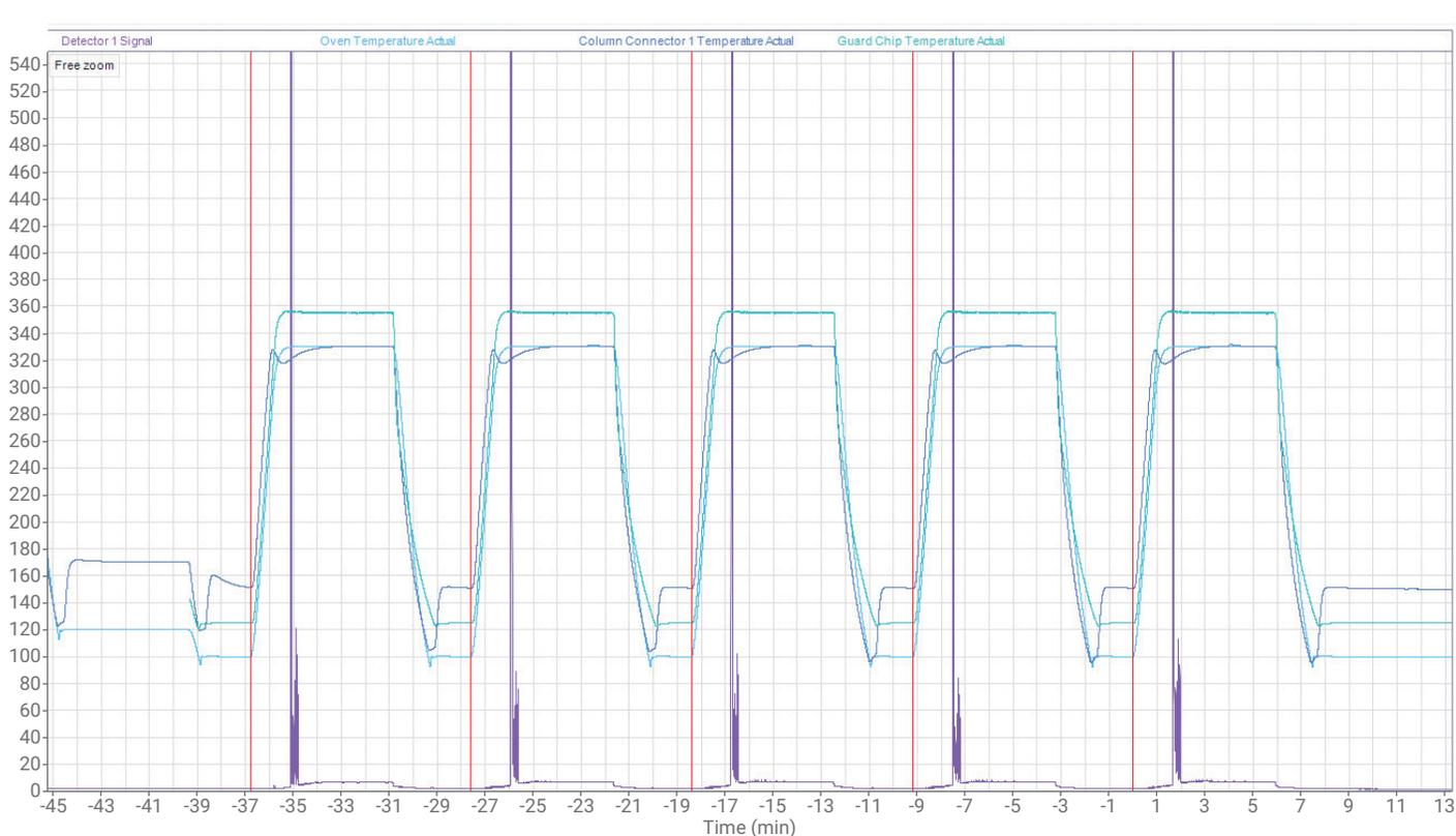
**Figure 1.** Thermal cycling profile of an J&W VF-5ms Intuvo GC column from 100 to 330 °C at 250 °C/min.
