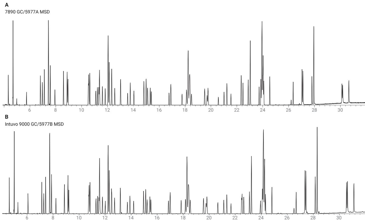
**Figure 6.** Overlaid chromatograms of the SVOC test mix using a 7890B GC with a 5977A MSD (A) and an Intuvo 9000 GC with a 5977B MSD (B).
