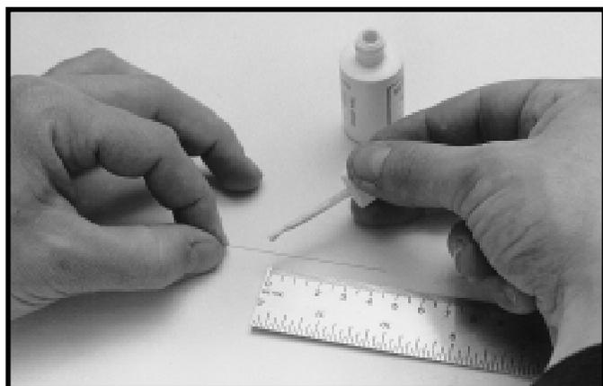
Once these insertion distances are marked, install the column in the injection port. Before completing the hook-up to the detector, turn on the carrier gas flow to purge the column. Typical head pressures for various column IDs and lengths are given in Table 1. You will later fine-tune these tentative settings.
