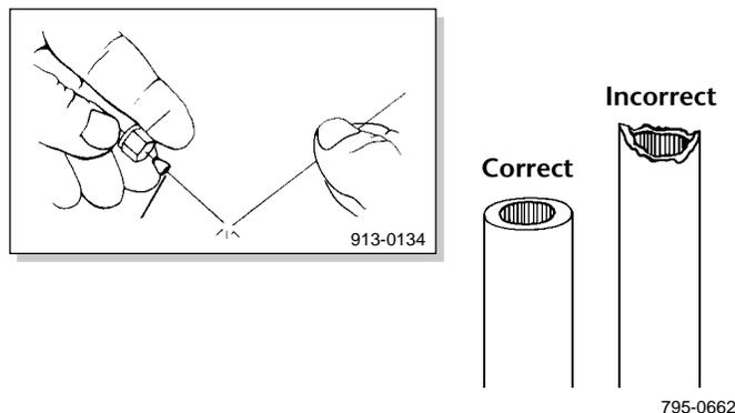
When installing a fused silica column in the injector port and detector, follow the instrument manufacturer's recommended insertion distances. Otherwise, column performance may be affected. Use typewriter correction fluid or a felt-tipped pen to mark the correct distances on the fused silica tubing (Figure C).
