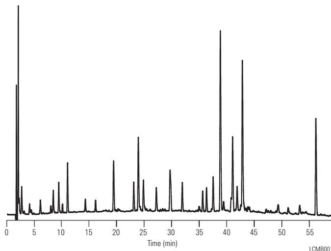
This example of a tryptic digest separated on a MicroBore column demonstrates the high sensitivity and resolution possible with 1.0 mm id columns.
