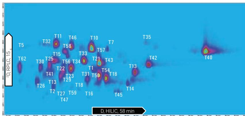
LCxLC contour plot for the analysis of the tryptic digest of trastuzumab generated with MS total ion count data. The two dimensions, HILIC in the first and RP in the second, had good orthogonality for this analysis.
