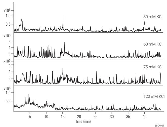
Tryptic digest of bovine serum albumin (BSA). The base peak chromatograms show a selection of fractions from a 2D HPLC separation. Single chromatograms represent peptides from BSA eluting at a given salt concentration followed by enrichment and reversed-phase chromatography.
