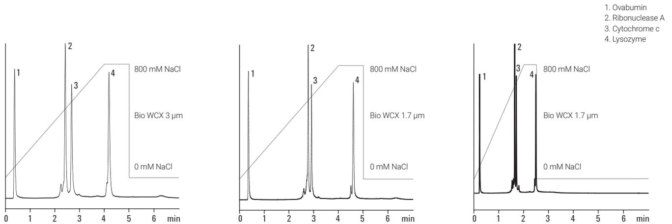
**Left and middle:** Protein separation on a Bio WCX 3  $\mu$ m column versus a Bio WCX 1.7  $\mu$ m column (flow rate 1.0 mL/min).
