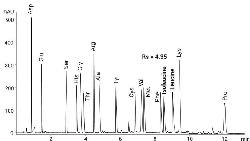
Ultraviolet chromatogram of amino acids from protein hydrolysate. The resolution between leucine and isoleucine is 4.35, which easily meets the European Pharmacopoeia requirement that resolution be greater than 1.5. [European Pharmacopoeia 9.0 (2.2.56) Amino Acid Analysis.]
