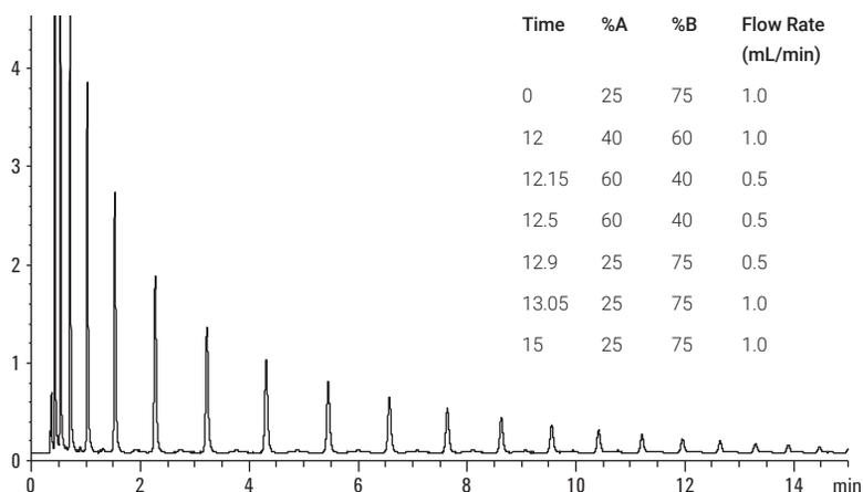
This analysis uses the Agilent dextran ladder standard, together with an AdvanceBio Glycan Mapping column to correlate retention times of unknown glycans.
