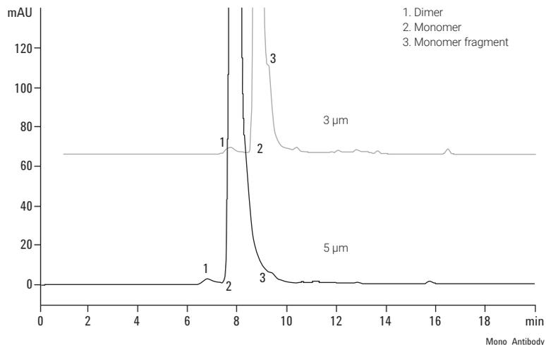
The 3 µm column gives higher definition of the fragmentation plan.
