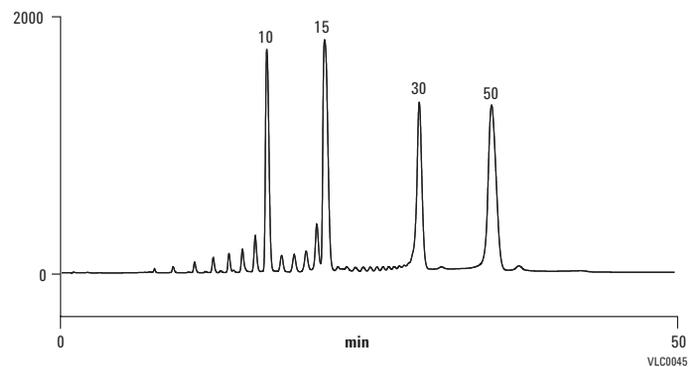
High-resolution separation of poly-t-oligonucleotide. With the gradient used here, baseline separation of the n-1 from n was easily obtained up to the 15-mer.
