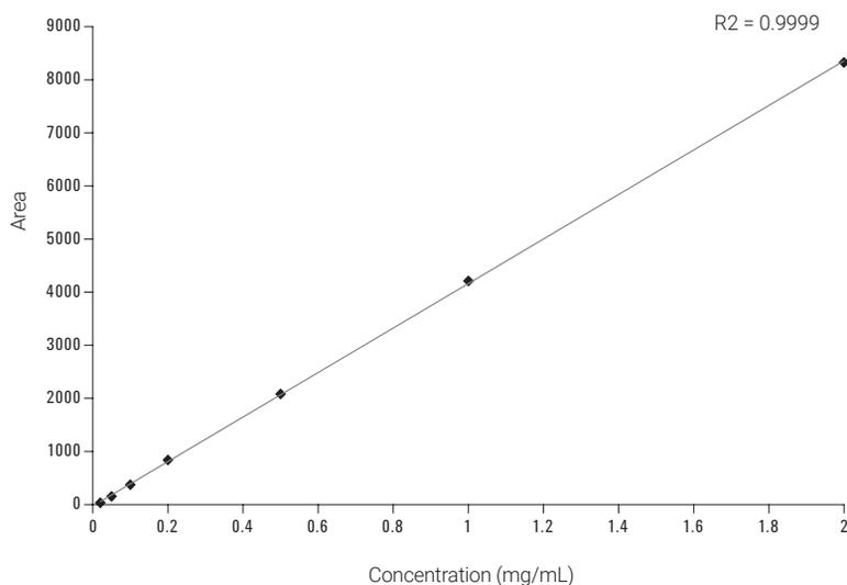
Calibration curves of modified humanized Trastuzumab (panel A: 0-2 mg/mL, and B: 25-200 mg/mL)
