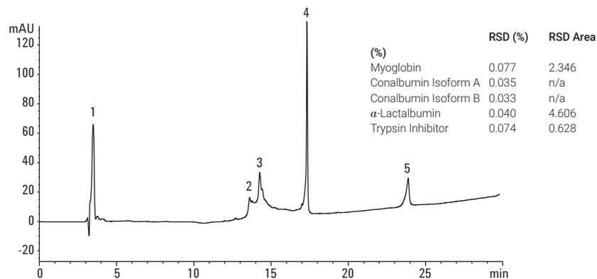
Figure 3. Protein separation by AEX by a linear gradient using 1 M [(CH<sub>3</sub>)<sub>4</sub>N]Cl as eluting salt.
