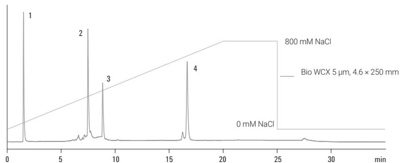
Protein separation on a Bio WCX 4.6 x 50 mm, 3  $\mu$ m column versus a Bio WCX 4.6 x 250 mm, 5  $\mu$ m column (flow rate 1.0 mL/min). Faster analysis times were achieved through smaller particle size and shorter column length—samples eluted from the longer column in 17 min, and in just 12 min from the shorter column.
