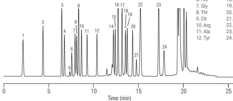
This high resolution separation of 24 amino acids is achieved in 18 minutes. If the Rapid Resolution 4.6 x 75 mm Eclipse AAA column is selected, these amino acids are resolved in 9 minutes.
