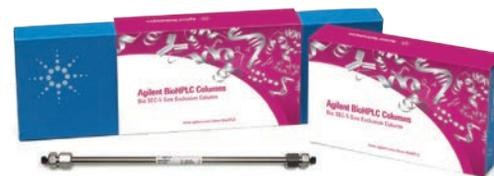
For large biomolecules and samples with components of multiple molecular weights, Bio SEC-5 columns are an ideal choice. They are packed with 5 µm silica particles coated with a proprietary, neutral, hydrophilic layer for maximum efficiency and stability, with six different pore sizes to provide optimum resolution over the molecular weight range.
