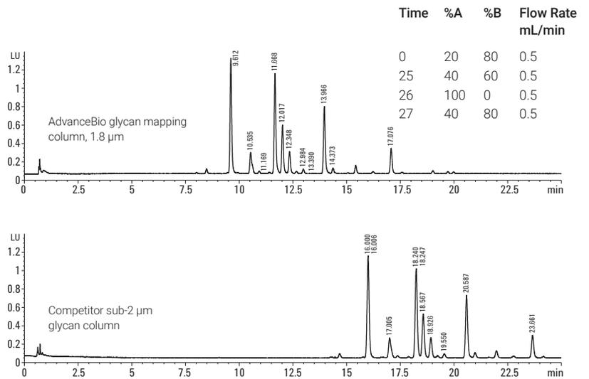
The AdvanceBio Glycan Mapping column delivers better resolution, narrower bands, and higher peak capacity than the non-Agilent sub-2  $\mu\text{m}$  column in a 2.1 x 150 mm configuration.
