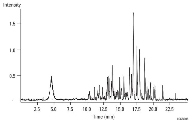
A ZORBAX nano HPLC column, 0.075 mm id, is used for high-sensitivity LC/MS analysis of a protein digest sample.
