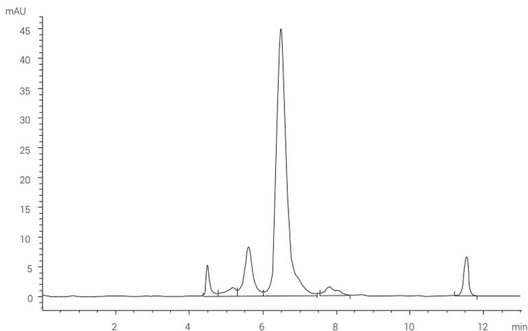
High-resolution separation of an IgG sample, showing the monomer, aggregates, and degradation products.
