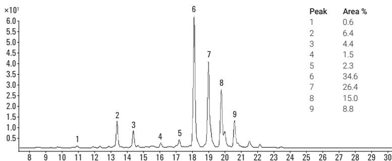
The N-glycans cleaved from fetuin using PNGase F were analyzed after 2-AB derivatization using UHPLC –FLD. The peak assignment by MS shows that the N-glycans cleaved from fetuin are complex biantennary and triantennary glycans containing N-acetylneuramic acid (NeuAc) but no fucose. Fetuin 2-AB N-glycans analyzed using HILIC-UHPLC with peak assignments determined by MS.
