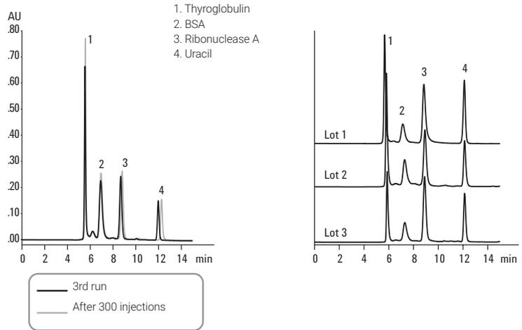
The four-protein mixture shows excellent retention time reproducibility over 300 injections and on three columns from different manufacturing lots.
