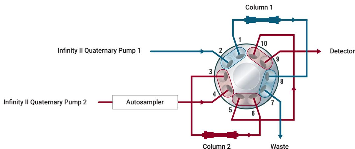
A schematic showing the valve arrangement required for offline column regeneration as would be used for mAb charge variant analysis using the 1260 Infinity II bio-inert LC, and two Bio MAb PEEK, 2.1 x 250 mm, 5  $\mu$ m columns.
