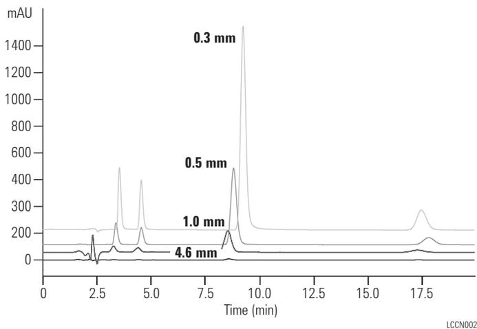
Sample-limited applications require capillary column dimensions to minimize on-column sample dilution and to enhance sensitivity. The 0.3 mm capillary in this example provides 100 times more sensitivity than the standard 4.6 mm column. Agilent nanobore (0.1 mm to 0.075 mm id) columns can provide up to 2,000 times more sensitivity for your most limited sample applications.
