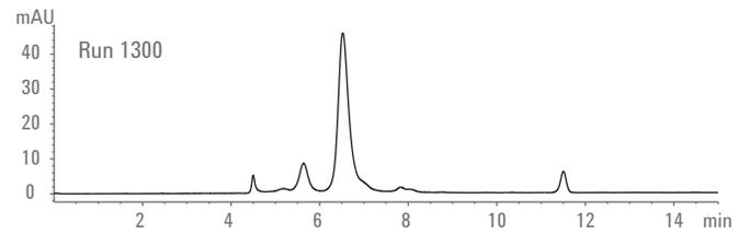
The profile of an IgG sample did not change—even after 1300 injections. Resolution factors and quantitation of the IgG monomer and dimer also remained within working range throughout the column lifetime.
