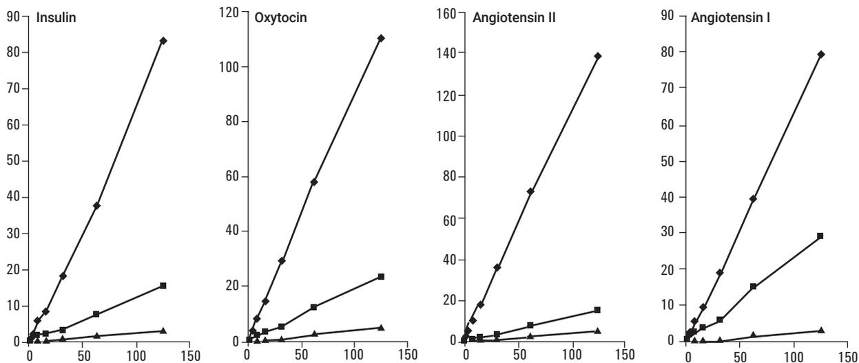
Standard curve data-point graphs on PLRP-S columns. Reduced column internal diameter reduces the limit of detection and enables quantitation of lower amounts of sample.
