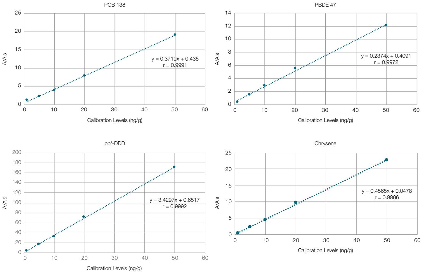
Figure 3. Calibration curves for PCB 138, PBDE 47, pp'-DDD, and chrysene (1–50 ng/g)
