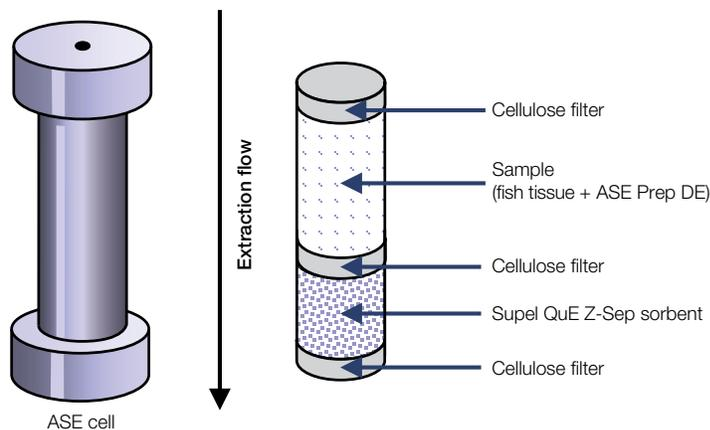
Figure 2. Extraction cell schematic
