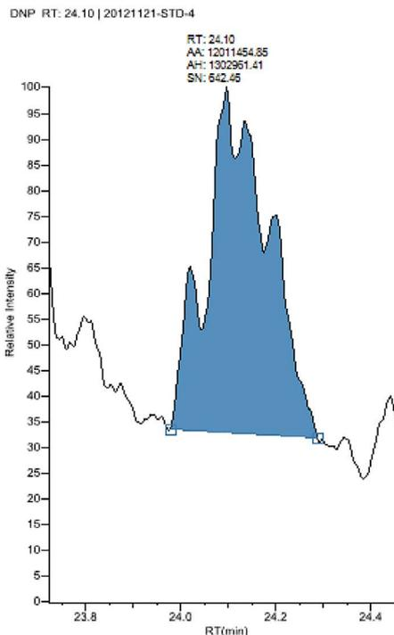
Figure 9. Quantitation peak of the unresolved DNP isomers over a set retention time range using the TraceFinder software (extracted mass 149  $m/z$ )
