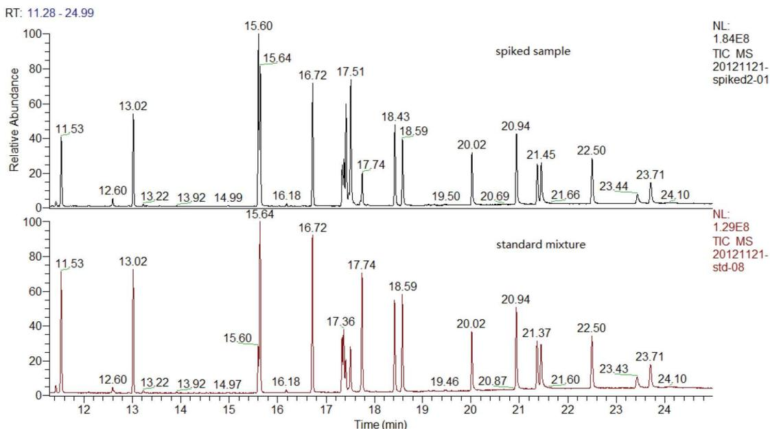
Figure 1. Chromatograms of a spiked sample at 0.8 mg/L (top) and of the mid-level standard mixture run (bottom)
