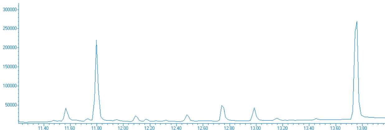
Figure 1: Total Ion Chromatogram of a 50ppt Geosmin and 2-Methylisoborneol Standard
