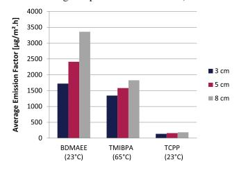
Figure 6. Emission factors [µg m<sup>-2</sup> h<sup>-1</sup>] of three opencell samples with three different thicknesses but the same surface area at 23°C or 65°C.
