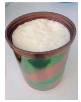
Figure 3. Custom-made coring tool and sample of the SPF open-cell foam (left) and the coring tool together with the sample, the surface at the top, placed into the one Liter container (right).
