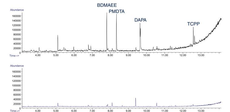
Figure 5. Lowest level SPF standard (25 ng per TD tube, top) compared with the background of the DHS Large one liter container the coring tool inserted (65°C, 1 liter sampling volume, bottom chromatogram).
