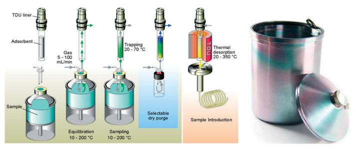
Figure 4. Automated micro-scale chamber method steps for a surface emission sample (left) with one liter DHS containers, made of electro-polished stainless steel and an inert surface coating (right).
