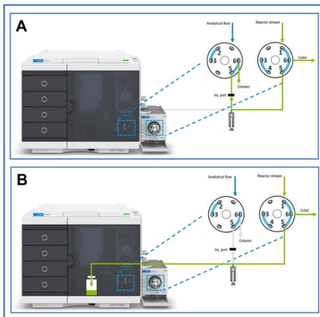
**Figure 1.** Schematic of the Agilent 1260 Infinity II Online Sample Manager and respective valve configuration enabling: (A) Direct injections from the external reactor sampling interface. (B) Sample handling for dilution/quenching prior to injection.
