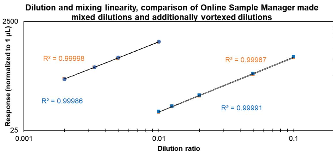
**Figure 7.** Determination of dilution and mixing linearity for dilutions made by the Agilent 1260 Online Sample Manager including mixing (orange series) and after an additional vortex step (blue series).
