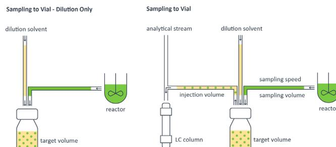
**Figure 3.** Schematic of the possible dilution/quenching of the reactor sample into a vial with subsequent analysis controlled by the Agilent Online LC Monitoring Software.
