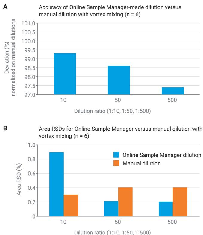
**Figure 5.** A comparison of areas from three dilution series prepared automatically by the Agilent 1260 Online Sample Manager and manually. (A) Accuracy of the automated dilutions with the Online Sample Manager compared with handmade dilution. (B) Area RSD values of the Online Sample Manager and manually prepared dilutions.
