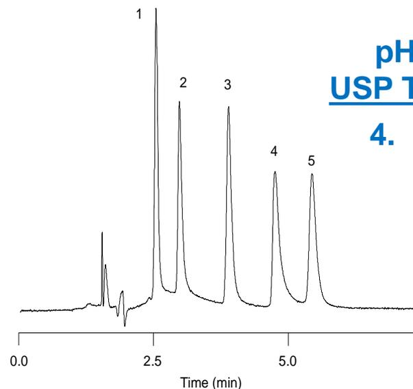
Tip: Reducing mobile phase pH reduces interactions with silanols and peak tailing.
