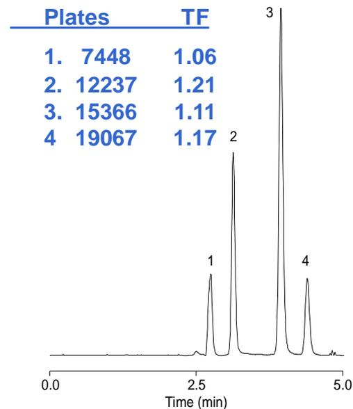
Column: StableBond SB-C8, 4.6 x 250 mm, 5 µm
