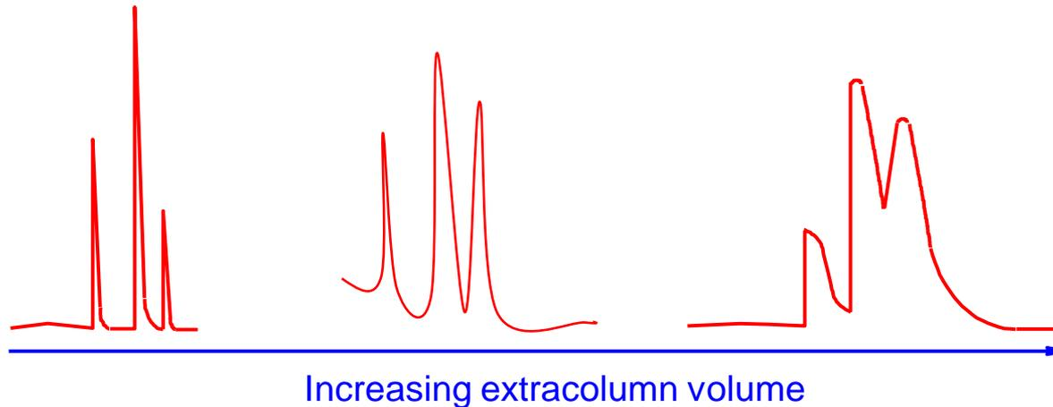
Use short, small internal diameter tubing between the injector and the column, and between the column and the detector.
