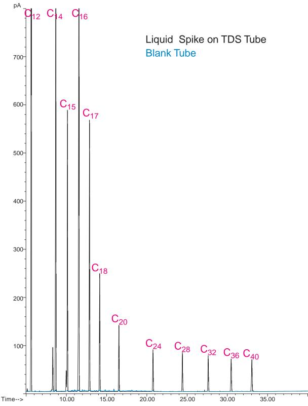
Figure 2. Overlay of 1ul liquid spike on TDS tube and following blank tube run.
