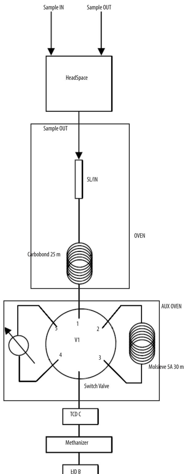
Figure 1: Schematic Diagram of DANI DGA 5 TOGA Analyzer
