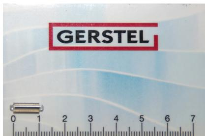
**Figure 1.** Twister PDMS stir bar, 1 cm length, 1 mm phase thickness.
