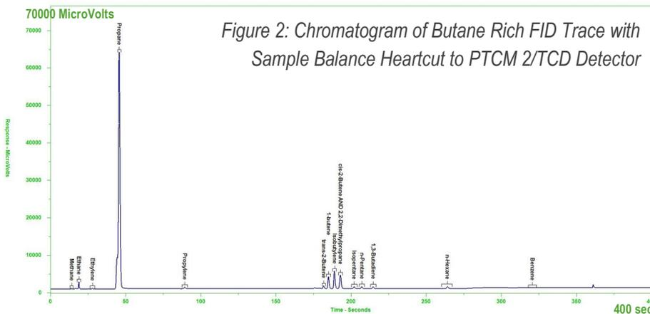
Figure 2: Chromatogram of Butane Rich FID Trace with Sample Balance Heartcut to PTCM 2/TCD Detector
