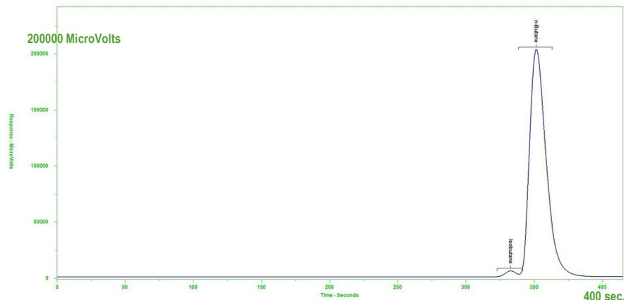
PTCM 2 contains a MXT-HS-Q resistively heated stainless steel capillary column and is operated in a delayed temperature programmed mode. This column provides separation of n-Butane and iso-Butane in Butane rich samples, and Propane in Propane rich samples (See Figure 3).
