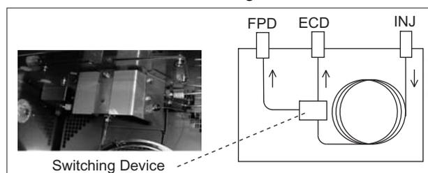
Fig. 1 Device Configuration for Detector-Switching Analysis
