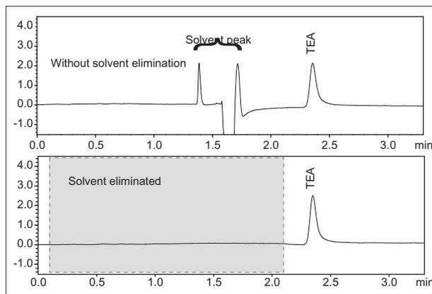
Fig. 3 Chromatograms of With and Without Solvent Elimination
